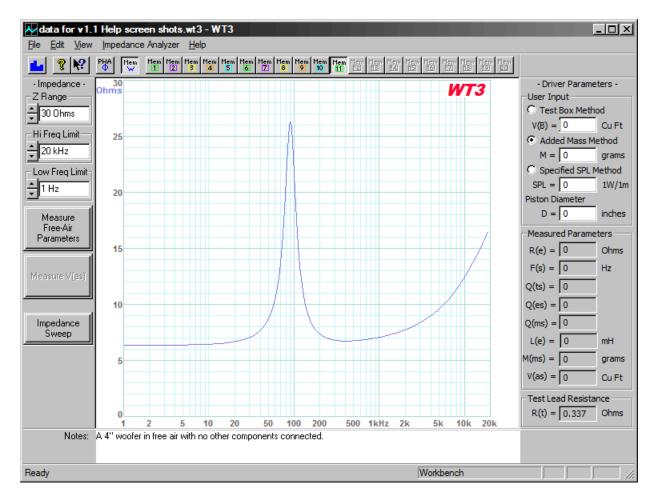
With a DC resistance of 5.5 Ohms this would most likely be considered to be an 8 Ohm driver. So let's set the resistor value to about 8 Ohms. Looking in my parts bin I see the closest values on hand are 5 and 10 Ohms. Let's use 10 Ohms so that we tend to under compensate. We'll select the capacitor value by starting too low and stepping up the capacitor until the impedance response looks about as flat as
